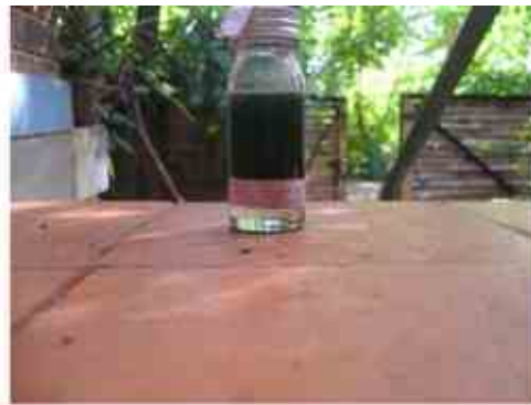
Fig 16 & 17: H 2 S Strip test bottle. Fill it with water. If the water turns black it needs to be treated
