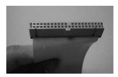
Check if the HDD jumper is set to master and any other device sharing the same cable is set to slave.
