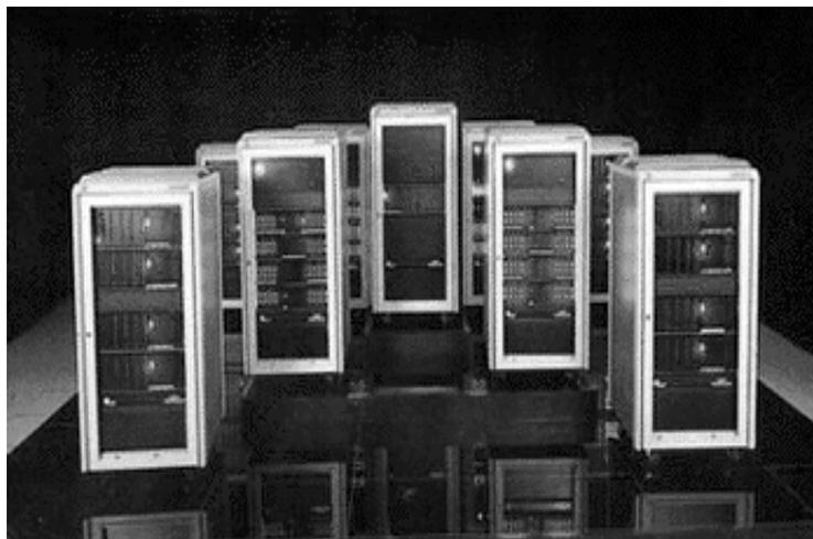
**Super Computer:** A computer with lots of processors, ALUs (Arithmetic logic unit), Memory (RAM), etc. Usually in scientific research work. Capability of 14,000 micro computers.
